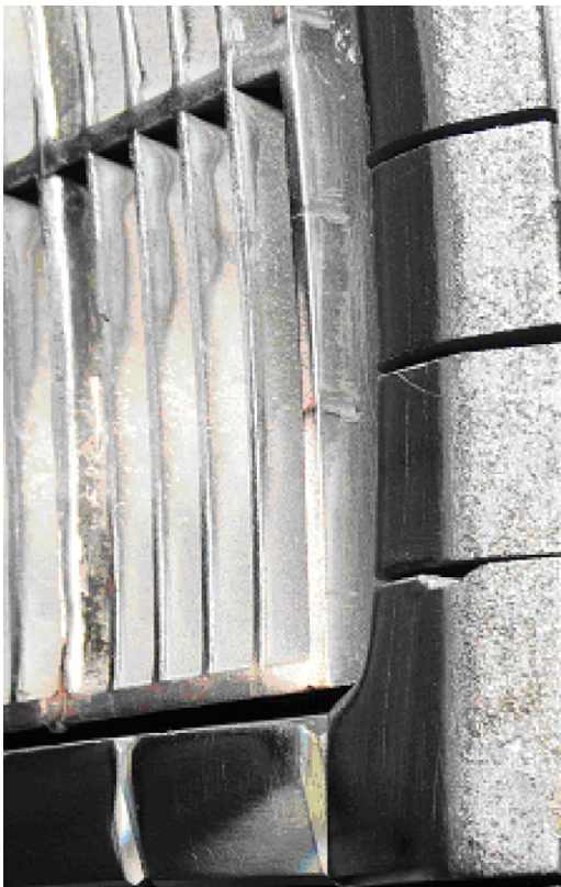
Fig. 6. Photo of a waveguide row on one LHCD launcher. A poloidally asymmetric heat pattern is observed. Stronger heating is observed in the upper part of each waveguide row.
